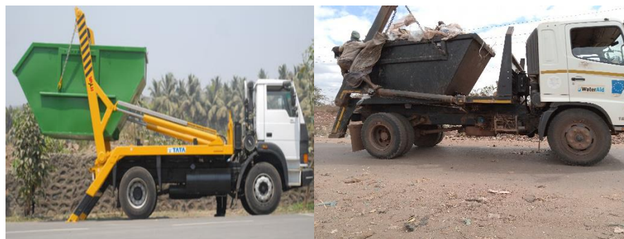
Figure 8: SW Skip Carrier Vehicles picture source: Field pictures at Lilongwe City Dump Site
