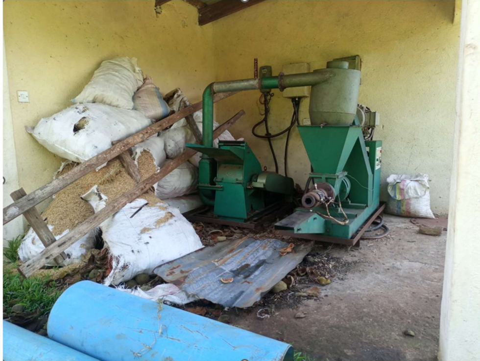
Figure 1-15. A photo showing a briquette making machine with some feedstock at Bondo 3.
