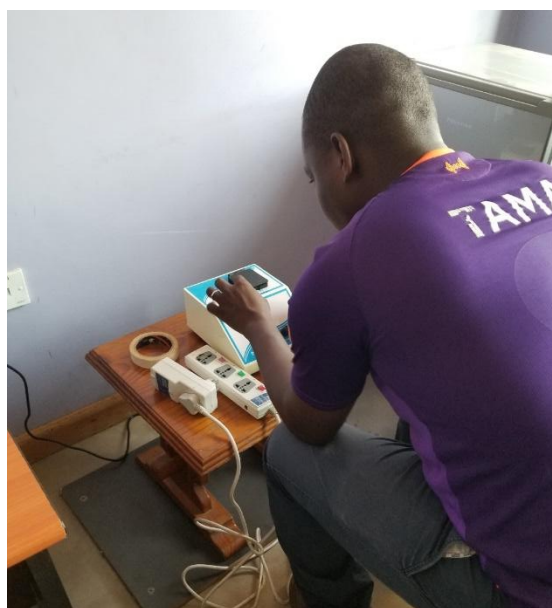
Figure 3-8: Water quality officer setting up the turbidity meter
