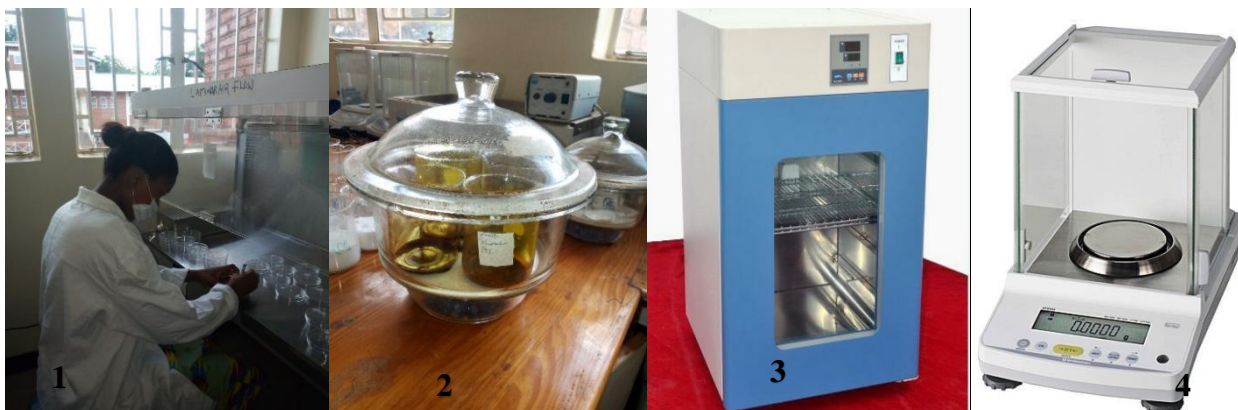
1 = Laminar flow, 2 = Desiccator, 3 = Oven and 4 = Analytical balance
